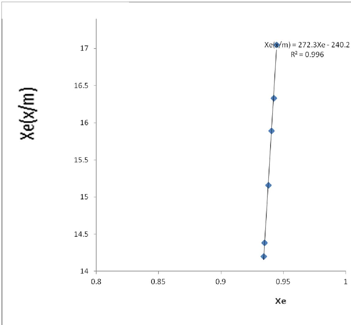
**Figure 2:** Langmuir isotherms for impurities in sunflower oils on recycled Kajansi clays leached in 20% acid.
