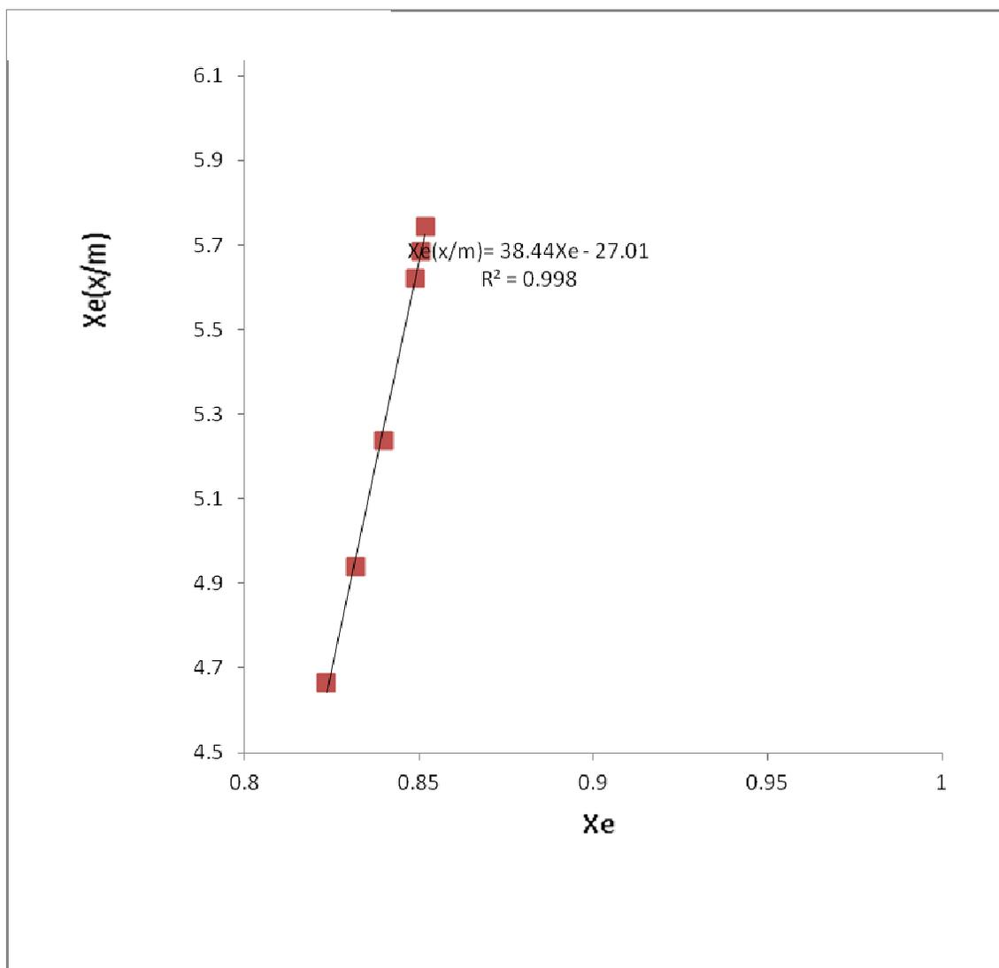
**Figure 1:** Langmuir isotherms for impurities in sunflower oils on recycled Chelel clays
