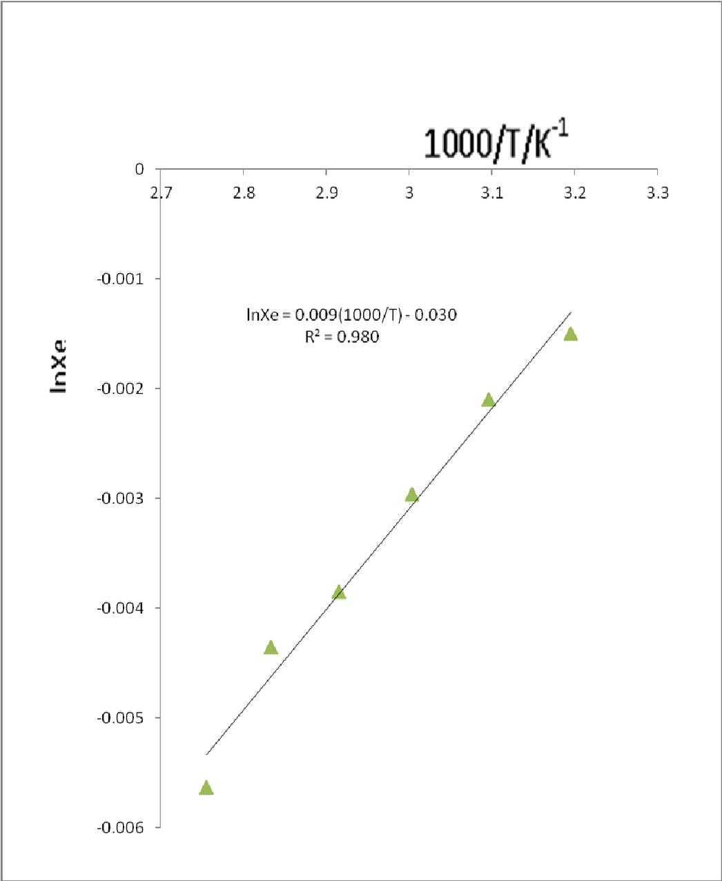
**Figure 3a:** Freundlich isotherm for impurities in cotton oils on recycled Chelel clay leached in 10% acid
