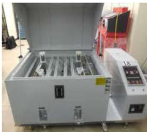
Figure 4: Generally, the specimens are opened to fine fog of salt water at 35 °C temperature. The concentrated solution varies based on the material to be checked.
