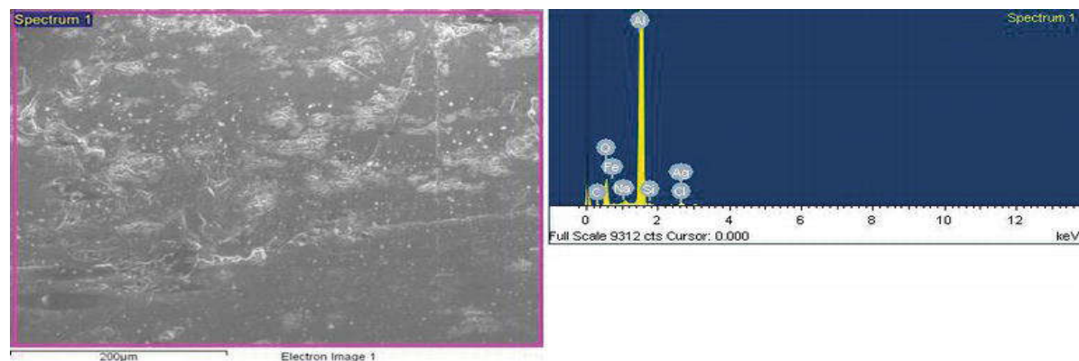
Figure 8: SEM/EDS spectra of corroded aluminium 356 in the presence of FG [47].
