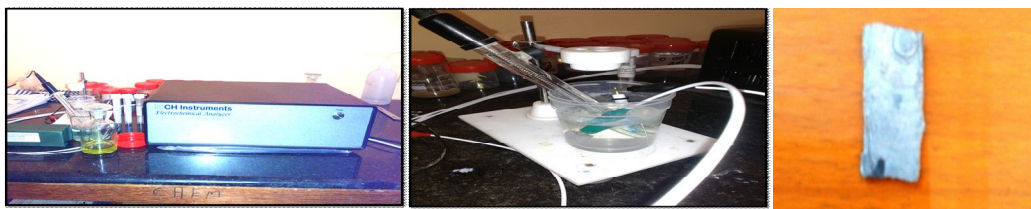
Figure 1: Experimental set up for potentiodynamic and EIS studies
