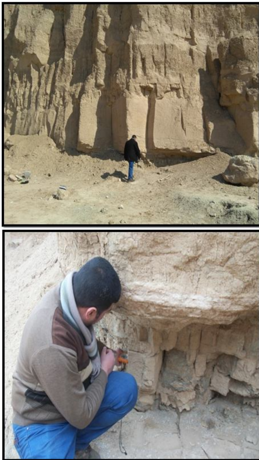
Figure 7: Sandstone rocks in study area Injana formation shows fractures attitude measured (dip and strike)
