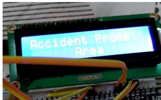
Fig. 7 – System displaying warning in when the vehicle enters an accident-prone area
