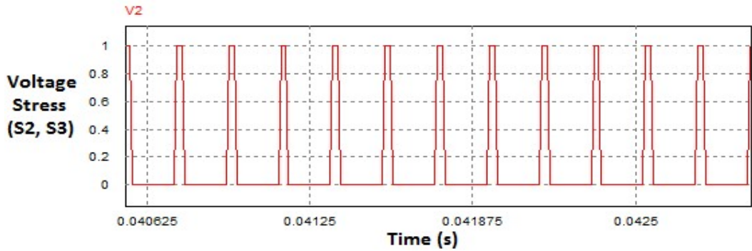
Figure 5.2.: Voltage stress across switch S2 and S3 (symmetrical source)
