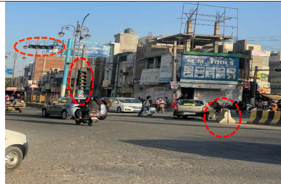
Fig. 2 shows the blackspot location of Dabra Chowk which shows that signal lighting not working, no crossing available, no traffic police for manual guiding, and the brigades are not properly used.
