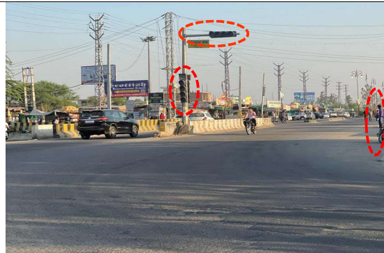
Fig. 3 shows the blackspot location, Azad Nagar which shows that signal lighting is not working in Azad Nagar, there is no pedestrian crossing, no road marking, and improper roadside parking.
