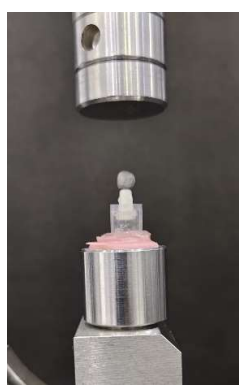
Fig 3b – Cyclic loading of Ti Implant PEEK abutment at 0 degree
