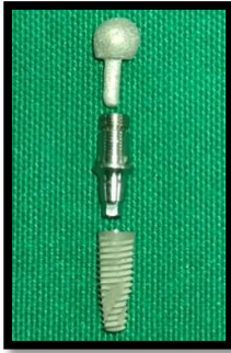
Fig 2a – load Adapter with Ti Implant Ti abutment
