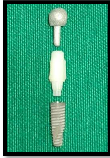
Fig 2b – load Adapter with Ti Implant PEEK abutment
