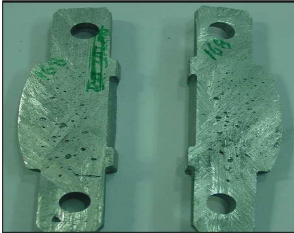
Figure 4: Cut section Porosity Level-4
