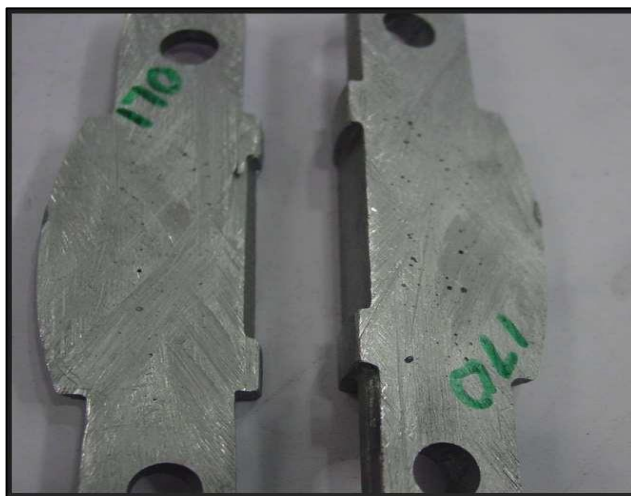
Figure 3: Cut Section Porosity Level-3
