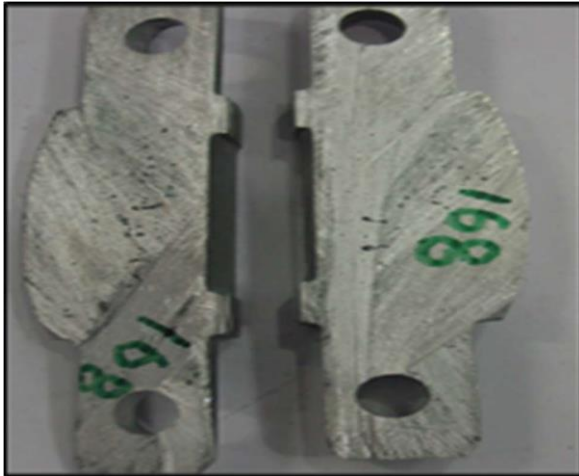
Figure 2: Cut Section Porosity Level-2
