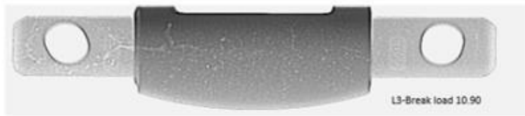
Figure 12: Porosity Level 3 Break load 10.90 KN
