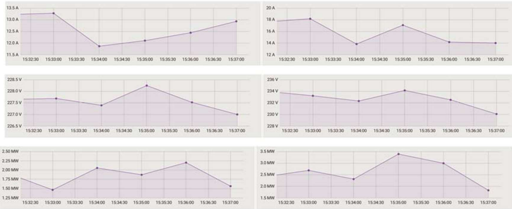
Figure 23: Monitoring voltage, current and power in the proposed residential building with DC supply
