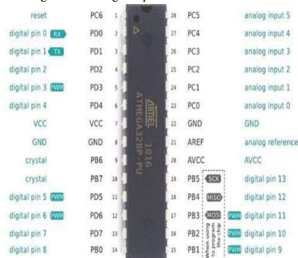
Figure 3: Pin diagram of Atmega328p microcontroller
