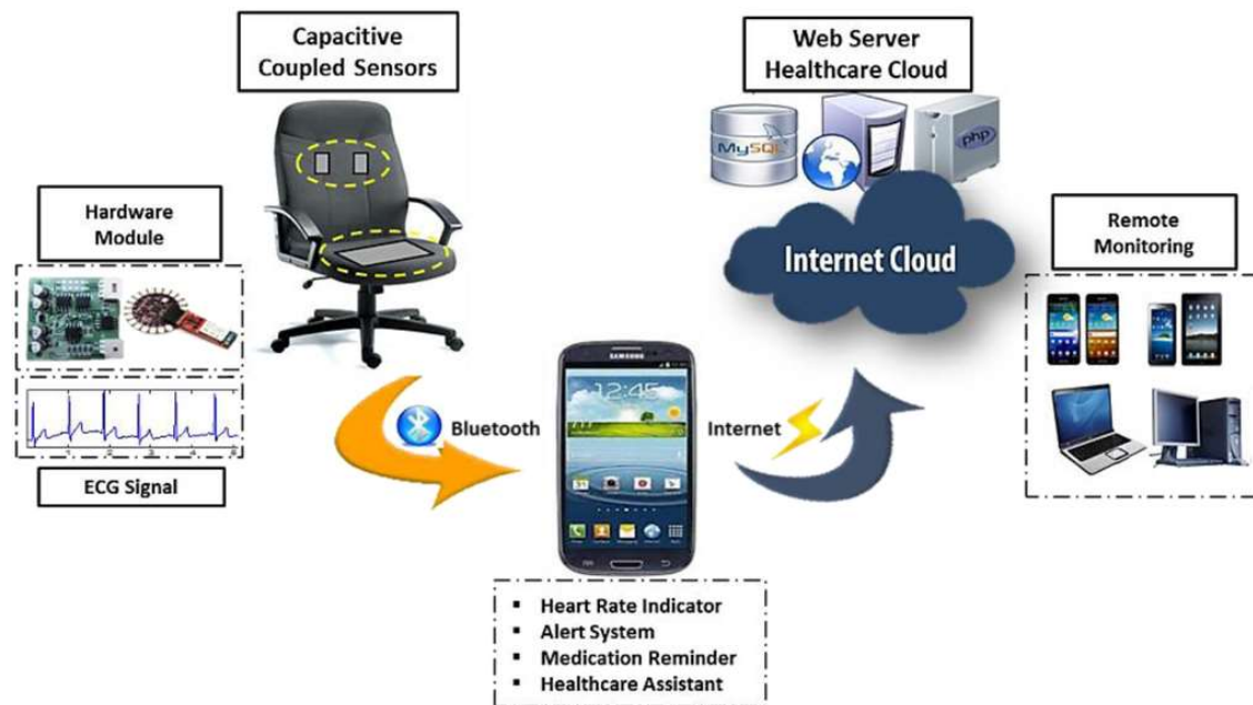
Figure 3: A noncontact electrocardiogram (ECG) monitoring system that incorporates cloud computing, a mobile device, and a data gathering module is designed for use in healthcare settings that prioritise mobility and accessibility [12].
