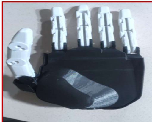
Figure (5): The additive wrist for the original system
