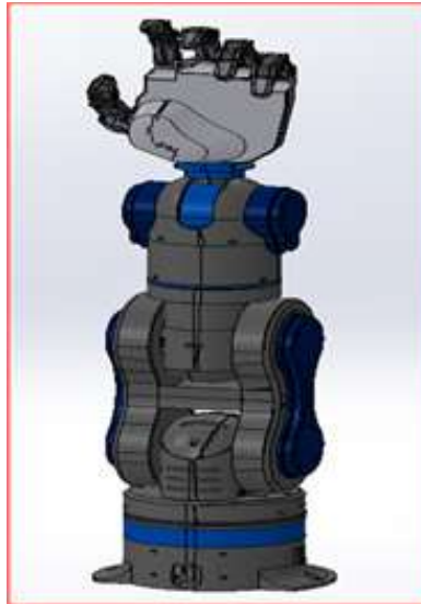
Figure (1): Complete assembly Thor robotic arm components design CAD model
