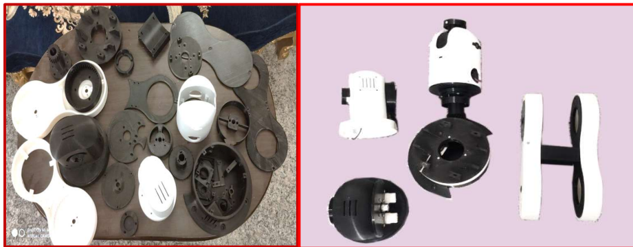
Figure (4): components that are printed as well as incomplete joint assemblies.
