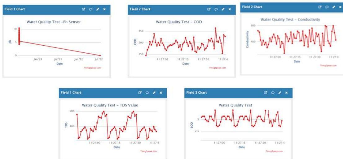
Figure 9: Visualization Display of Varying Parameters with Time in ThinkSpeak Cloud
