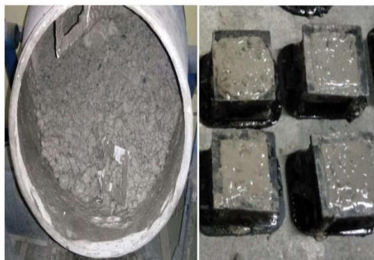
Figure 3: Casting of GPC specimen
