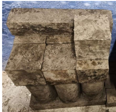
Figure 4: Ambient curing of GPC specimen
