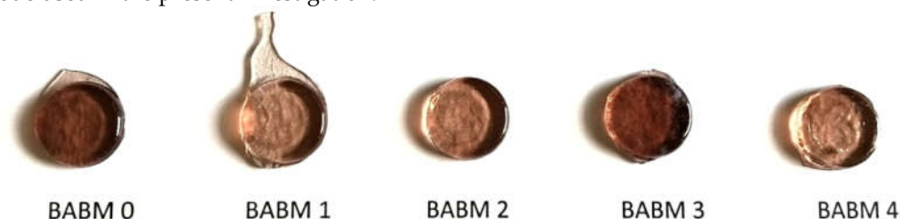
Figure 1: Images of prepared glass samples of BABM
