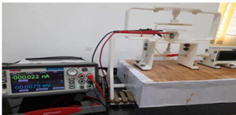
Figure 1: Measuring TENG output with a Keithley 2450 sourcemeter
